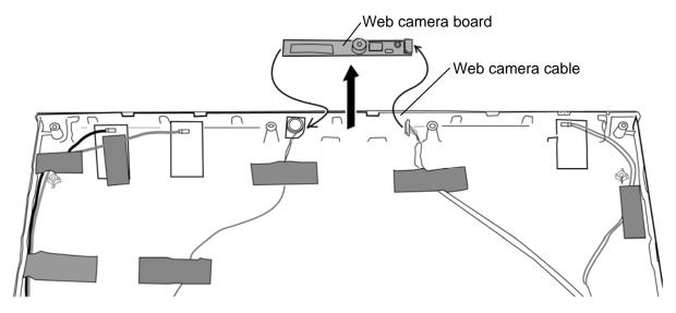
Figure 4-57 Removing the web camera board
